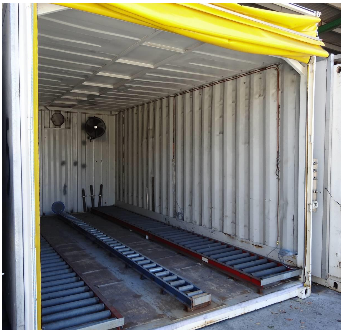
Figure 3 Typical fumigation chamber used by third-party quarantine approved premises
